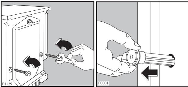
Remove the polystyrene block from the bottom of the machine and release the two plastic bags. Very carefully slide out the left polythene bag, removing it towards the right and then downwards.
