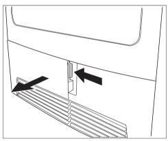
1. Open door in plinth: To do this, press the release button on the right and open the door in the plinth to the left.
