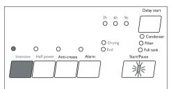
2. Press the *Intensive* button - the LED above is on.
