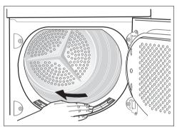
2. Use a damp hand to clean the micro- fine filter, which is built into the lower part of the loading aperture.
