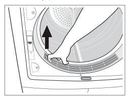
After a period of time, a patina due to detergent residue on laundry forms on the filters. When this occurs, clean the filters with warm water using a brush. Remove the filter from the door pulling it out. (It can be positioned with the locating spur facing to the left or to the right).
