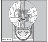
With the spanner provided unscrew and remove the central rear bolt **A**. Slide out the relevant plastic spacer.
