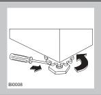
After having levelled the machine, tighten the lock nuts.
