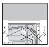
Set the hose correctly by loosening the ring nut.
