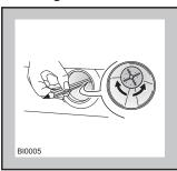
Refit the cap on the emergency emptying hose and place the latter back in its seat.
