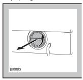
Remove any objects from the pump impeller by rotating it.
