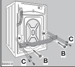
Remove the bracket **D**, refit the six smaller bolts **C**.
