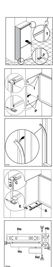
Place guide (Ha) on the inside part of the furniture door, up and down as shown in the figure and mark the position of external holes. After having drilled holes, fix the guide with the screws supplied.
