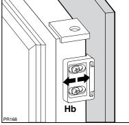
If the appliance is fixed to the side of the kitchen unit, simply slacken the screws in fixing brackets (E), move the brackets as shown in the figure and retighten the screws.
