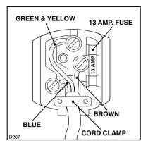
Connect the Green and Yellow (earth) wire to the terminal in the plug which is marked with the letter «E» or the earth
