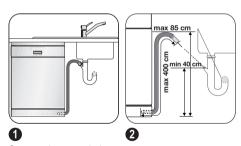
Connect the water drain hose to the sink spigot.
