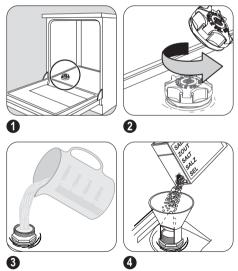
Fill the salt container with 1 litre of water (only the first operation).
