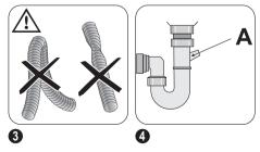
The internal diameter must not be smaller than the diameter of the hose
