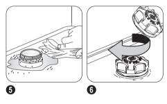
It is normal that water overflows from the salt container when you fill it with salt.
