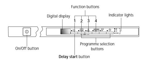
**Function buttons:** in addition to the selection of the washing programme and the delay start option, the following functions can also be set with the help of these buttons:
