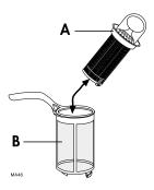
3. Turn the handle about 1/4 a turn anticlockwise and remove.
