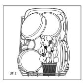
The two rows of prongs on the lower basket can be easily lowered to allow you to load pots, pans and bowls.
