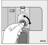
**1** Top up the rinse aid when the indicator light on the control panel illuminates.
