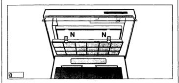
Always specify the hood model code number and serial number when ordering replacement filters. This information is shown on the registration plate located on the inside of the unit.
