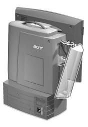
**Note:** When reinstalling the cable guise, arrange all the peripheral cables so that they run through the hole provided on the lower part of the cable guise.
