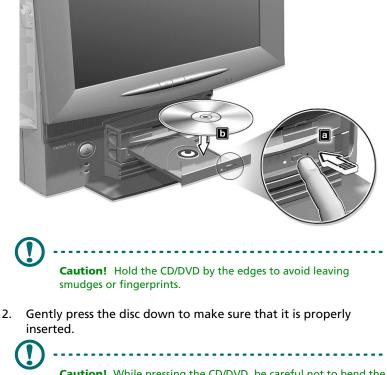
**Caution!** While pressing the CD/DVD, be careful not to bend the disc tray. Make sure that the CD/DVD is properly inserted before closing the disc tray. Improper insertion may damage both the CD/DVD and the CD-ROM/DVD-ROM/CD-R/W drive.
