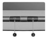
The two keys in the control panel which allow you to adjust the brightness setting of your LCD monitor are the following:
