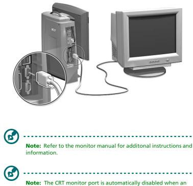
add-on VGA card is installed into the system. Connect the monitor to the VGA port instead.
