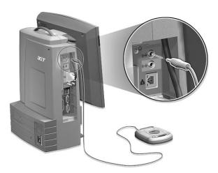
• other audio line-out devices: connect to the Line-out port (lime port) located on the left panel of your computer.
