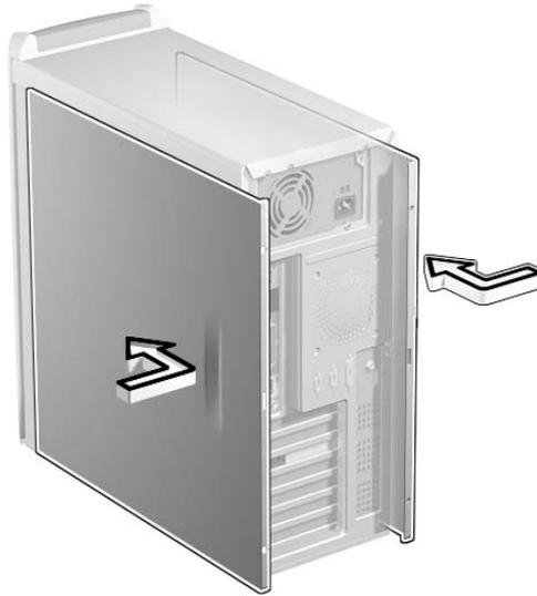
**2 Secure the side panels with the four screws you removed earlier.**
