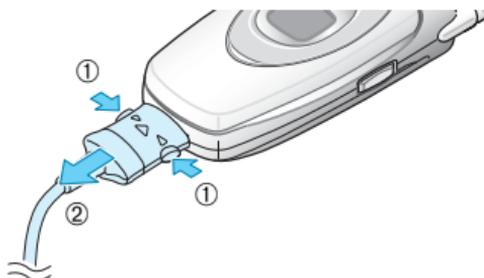
**Note:** You must unplug the adapter before removing the battery from the phone during charging; otherwise, the phone could be damaged.
