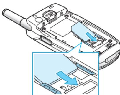
**Note:** When you need to remove the SIM card, slide it upwards, as shown, and take it out of the socket.
