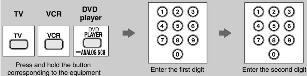
The remote control outputs the on/off signal. If the code is correct, the equipment turns on or off. If it doesn't, try entering another code.
