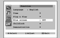
If no signal is being received or the signal is very weak, a blue screen automatically replaces the noisy picture background.
