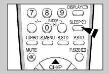
You can select a time period of between 30 and 180 minutes after which the television automatically switches to Standby mode by pressing the "SLEEP 🕙 " button.
