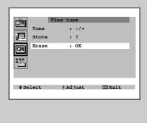
If the reception is clear, you do not have to fine-tune the channel, as this is done automatically during the search and store operation. If however the signal is weak or distorted, you may have to fine-tune the channel manually.
