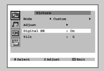
If the broadcast signal received by your television is weak, you can activate the Digital Noise Reduction feature to help reduce any static and ghosting that may appear on the screen.
