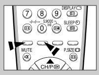
The various topics included in the teletext pages are color-coded, and can be selected by pressing the colored buttons on the remote control.
