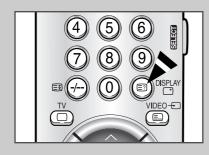
You can set the television's clock so that the current time is displayed by pressing the "DISPLAY" button. You must also set the time if you wish to use the automatic on or off timers.
