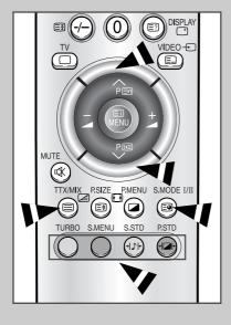
The various topics included in the teletext pages are color-coded, and can be selected by pressing the colored buttons on the remote control.
