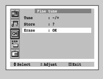
If the reception is clear, you do not have to fine tune the channel, as this is done automatically during the search and store operation. If the signal is weak or distorted, you may have to fine tune the channel manually.
