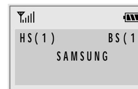
2. To turn the handset off, press and hold
