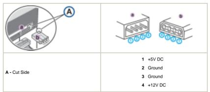
**Note:** An improperly connected power cable may cause trouble. Check the direction of the power connector and the incline side of the CD-R/RW drive before connecting.
