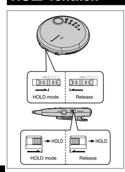
This function causes the unit to ignore short, accidental button presses. (The disc lid can still be opened and closed.
