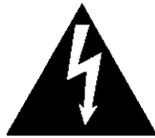
The lightning flash with arrow-head within a triangle is intended to tell the user that parts inside the product are a risk of electric shock to persons.
