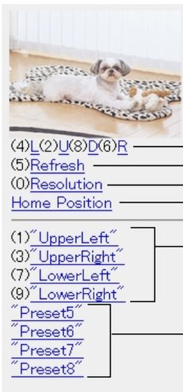
Pressing 2, 4, 6 or 8 on the mobile phones allows you to pan or tilt the camera in four directions: Left, Up, Down or Right.
