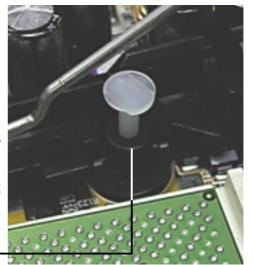
2. Open the retaining clips, place the heatsink on the CPU, then close and snap the clips into the locked position.
