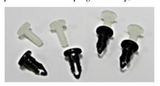
1. Mount the CPU as shown on page 27. Mount the *heatsink support braces* as shown on page 28 and insert the four black *plastic collars* from the top through to the bottom of the motherboard. Insert the white *plastic plugs* into the middle of the black collars and pop them firmly out the bottom of the motherboard.
