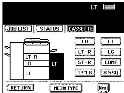
**9** Press the drawer key corresponding to that in which the paper size has been changed, then press the key of the paper size newly set.
