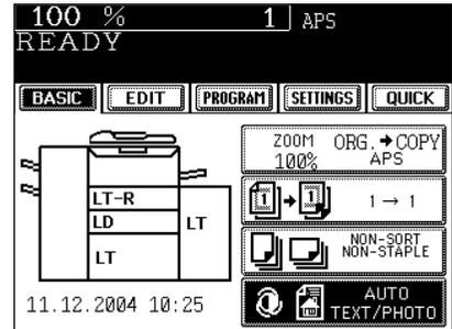
**4** Press either **(L)** or **(R)** key to adjust the copy density to the desired level.
