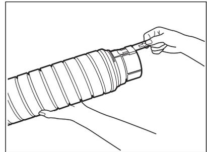
**5** Match the label (orange) on the machine with the shutter (orange) on the toner bottle, then insert the toner bottle to the end.
