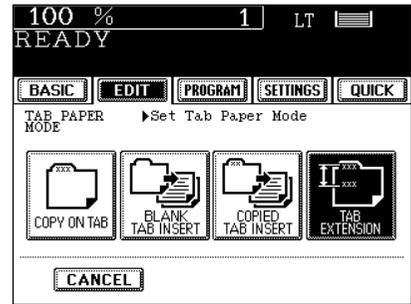
**3** Press the **CASSETTE** key (or the **BYPASS FEED** key), then adjust the tab extension (tab width) and the shift width then press the **SET** key.
