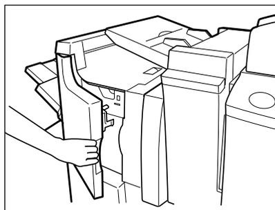
**2** Lower the blue lever in the stapler and slide out the staple cartridge.
