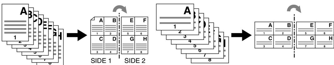
When a copy is turned with the line ——— as a pivot, originals are printed on side 2 (back face) as shown.
