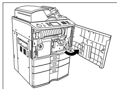
**2** Rotate the left end of the holder, then pull out the empty toner bottle with both hands as shown on the right.
