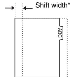
\* The shift width means the distance the image should be shifted when copied on the tab paper.
