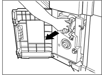
**7** **3** Pull out the grip of the saddle staple holder ① toward you and turn it ② 90° clockwise in the direction of the arrow.
