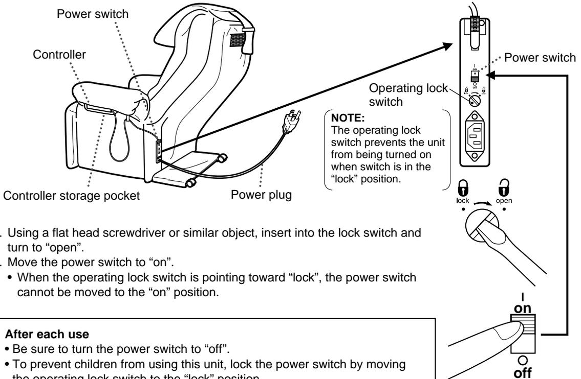
3. Using a flat head screwdriver or similar object, insert into the lock switch and turn to "open".
