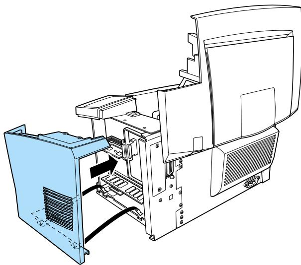
7. Fasten the side cover with the two screws.
