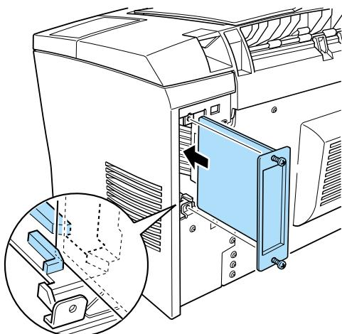
4. Secure the interface card with the two retaining screws.
