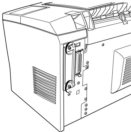
5. When you finish installing the option, plug in the power cable and reconnect the interface cables before turning the printer on.
