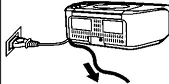
Extend and change the direction of the antenna lead.
