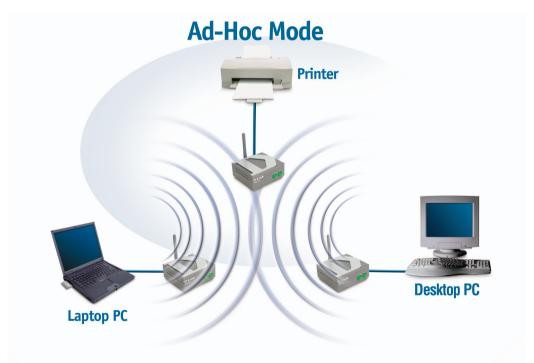
This example illustrates an **Ad-Hoc** setup. Simply connect the DWL-G810 (*refer to the Quick Installation Guide*) to your Ethernet-capable network device and you will be able to connect wirelessly with other devices also connected to DWL-G810's.
