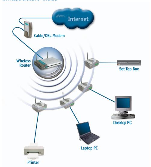
This example illustrates an **Infrastructure** setup. To connect the DWL-G810 to a wireless network with a wireless router or access point, please refer to the printed Quick Installation Guide included with the product. Web configuration is required to connect the DWL-G810.
