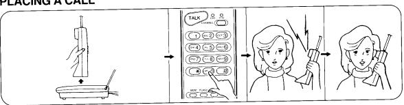
Lift the handset from the base unit, and press the TALK button. The CHANNEL LED lights.
