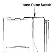
Set the TONE/PULSE switch located rear of the base unit for the type of service you have (tone or pulse). If you are not sure which type of service you have, do this simple test.
