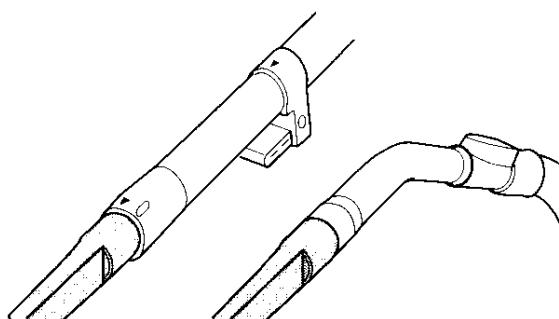
※Connect the crevice nozzle to the end of the extension pipe.
